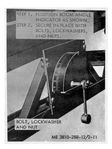
Figure 2-8. Crane boom angle indicator installation.
