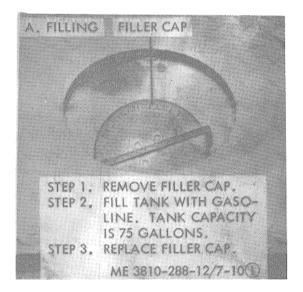
Figure 6-2. Fuel tank service (sheet 1 of 2).
