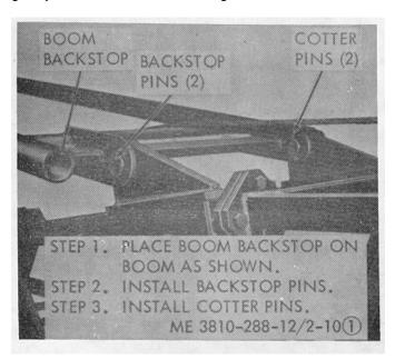
Figure 2-7. Boom backstop installation. (sheet I of 21.
